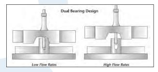
To maintain accuracy, the meter must be installed horizontally  $(\pm 10^\circ)$  in the direction of water flow. The Spectrum Jet 88DL and 88 DLT come with an integral test port on the outlet. Although regular maintenance is not required, the Spectrum Jet Model D meters have a top-loading measurement chamber for simple access without removing the meter from service. The chamber is bolted to the meter body and secured with a tamper seal.
