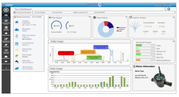
WaterScope<sup>™</sup> provides full details of your water consumption.
