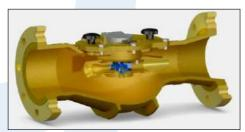
All bearing materials are fortified for minimal wear during high-flow stress. The impeller shaft utilizes tungsten tips to minimize wear and ensure long-term accuracy. The Spectrum Enduro meters come with integral flanges (either 6" or 8").
