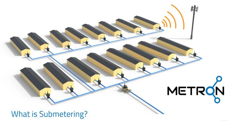
Simply put, submetering is where you put Metron's cellular water meters downstream of a single "master" meter which the water utility uses to measure the total water consumed by the property. You get to see the water consumption of the submeters by using WaterScope®, gaining insight into how the water is being used within the property. The water utility doesn't see the data from your submeters – they are for your use exclusively. There are many great applications for submetering.
